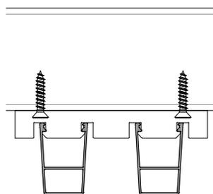
DETALLE ANCLAJE VIGA V-45 A ESTRUCTURA DE ACERO
